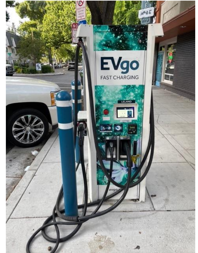
Three Connectors, one EVSE - CCS-1, CHAdeMO and Tesla
